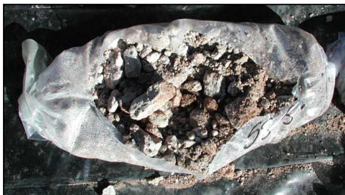
Soil extracted during drilling is closely examined and analyzed to provide information about the hydrology and geology of the site.
