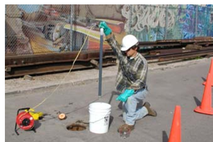
Sampling at the Site from a Monitor Well
